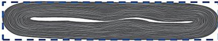
Conventional Wound Lithium-Ion Cell
